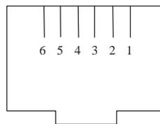
Figure 1 RJ11 plug (front view)
