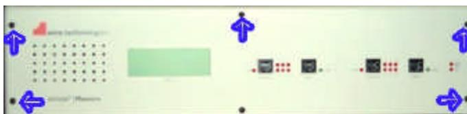
2. Rotate the **emutel™Maestro** 90 degrees. Now looking at the side panel of the **emutel™Maestro** as in Figure 2, remove the 4 screws indicated.
