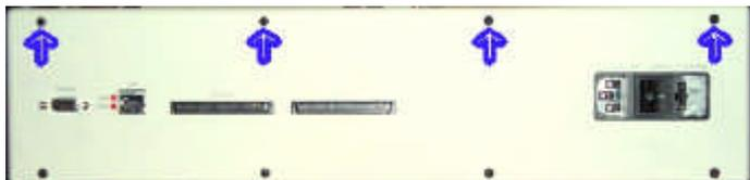
4. Rotate the emutel™Maestro 90 degrees. Now looking at the side panel as in Figure 2, remove the 4 screws indicated.
